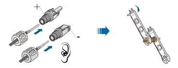
step 4 Check for polarity correctness.
