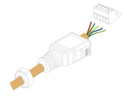
step 5 Strip 80 mm  $\sim$  90 mm of the cable jacked and 12 mm of the wire insulation.
