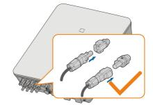
step 2 Ensure that the connectors are securely in place.
