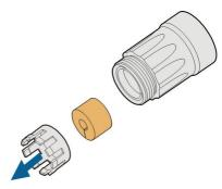
step 4 Insert the RJ45 plug into the front plug connector until there is an audible click, and install the rubber gasket.
