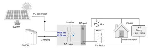
figure 8-26 DO Operation in Intelligent Mode
