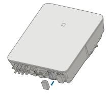
step 3 Align the Backup connector and the BACK-UP terminal and mate them together by hand until a "Click" is heard or felt.
