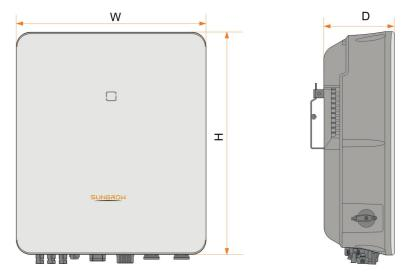
figure 2-2 Dimensions of the Inverter
