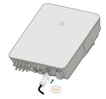
step 4 Pull all the lines outward to check whether they are firmly installed.
