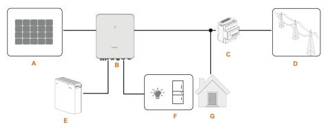
figure 2-3 PV Energy Storage System (PV ESS)
