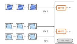
For SH10RT, if two PV strings are paralleled externally, the paralleled strings can be connected to PV2 or PV3 only, and the other one cannot be used to connect other PV strings.
