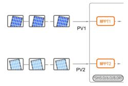
For SH10RT, each pair of PV terminals is corresponding to an independent PV string. PV input PV1 connect to MPPT1 and PV2, PV3 connect to MPPT2. For the best use of PV power, PV2 and PV3 should be the same in PV string structure, including the type, number, tilt, and orientation of the PV modules.
