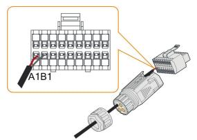
step 6 Pull the wires outward to check whether they are firmly installed.
