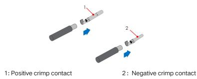
step 3 Lead the cable through cable gland, and insert the crimp contact into the insulator until it snaps into place. Gently pull the cable backward to ensure firm connection. Tighten the cable gland and the insulator (torque 2.5 N.m to 3 N.m).
