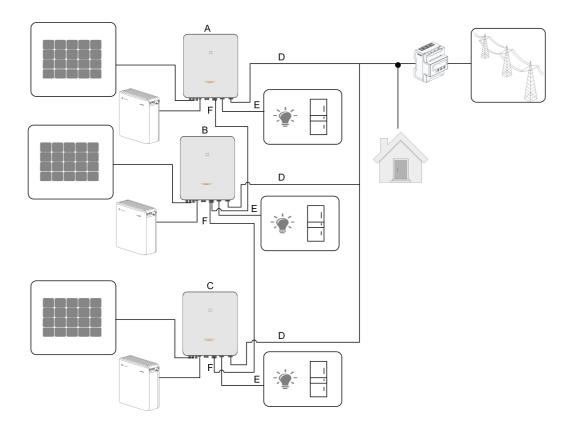
figure 2-4 Parallel PV ESS
