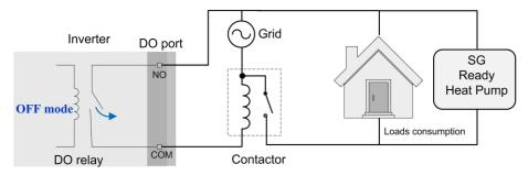
figure 8-25 DO Operation in Switch Mode
