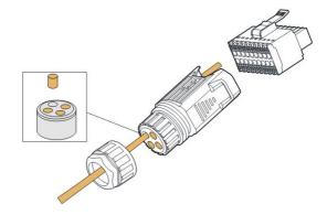
step 4 Remove the cable jacket and strip the wire insulation.
