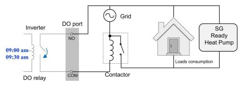
figure 8-24 DO Operation in Timing Mode
